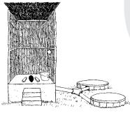
A water-seal trap, a platform, 1 or 2 deep pits, and a shelter. Best in places with deep groundwater and where people use water for anal washing after using the
