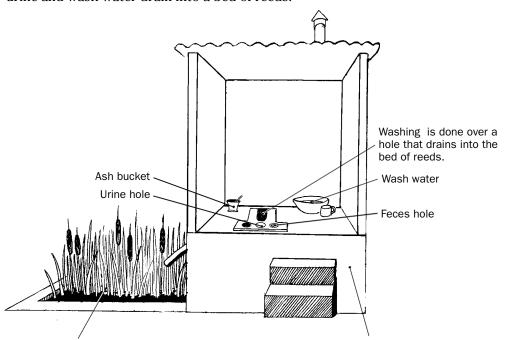
The plant bed where the wash water and urine go is filled with sand and gravel and planted with reeds or other local, non-edible plants. When the plants grow too big, they are cut back and thrown in the toilet.
